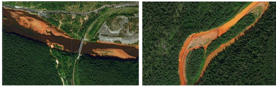
Fig. 4. High resolution images of rivers and sediments contaminated by acidic mine water in the Kizel coal basin (left – Kos'va; right – South Vil'va; modified from (Pyankov et al., 2021).
