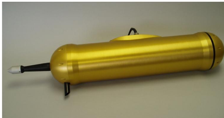
Figura 30 - Passive Cavity Aerosol Spectrometer Probe (PCASP)
