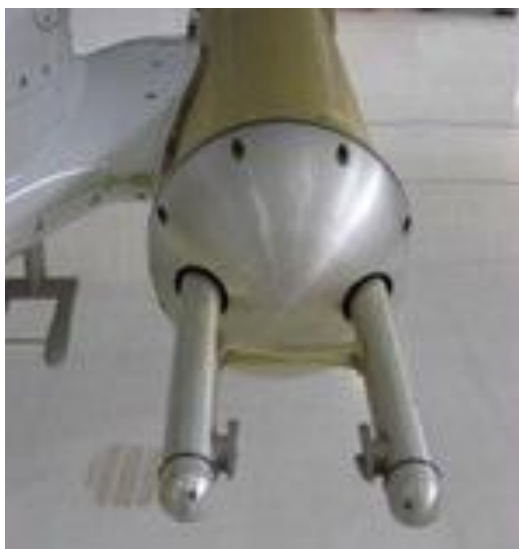
Figura 13 - Two Dimensional Cloud Probe (2D-C) instalada no HIAPER
