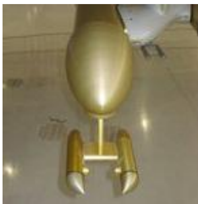
Figura 12 - CDP instalada no HIAPER
