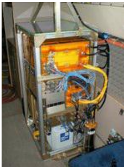
Figura 11 - Quantum Cascade Laser System (QCLS)
