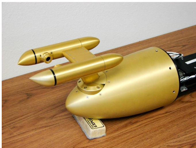
Figura 28 - Cloud Droplet Probe (CDP)
